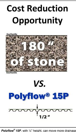
**Polyflow**<sup>®</sup> **15P**, with  $\frac{1}{2}$ " height, can move more drainage water per foot width than a layer of stone which is 1 ft. and 180" high. (Manning's equation used to calculate flow for the stone)
